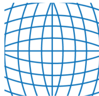
positive radial distortion "barrel"
